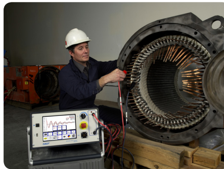
Surge testing a stator is safe with the Baker DX
